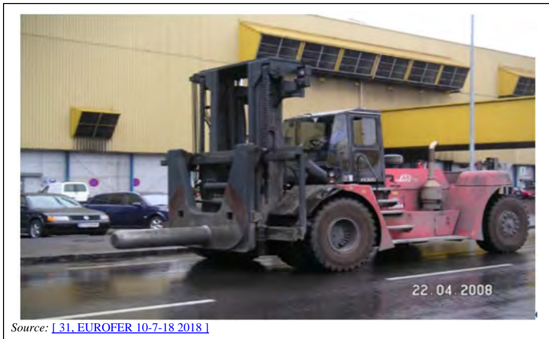
Figure 8.6: Piler with mandrels for coil manipulation and transport
