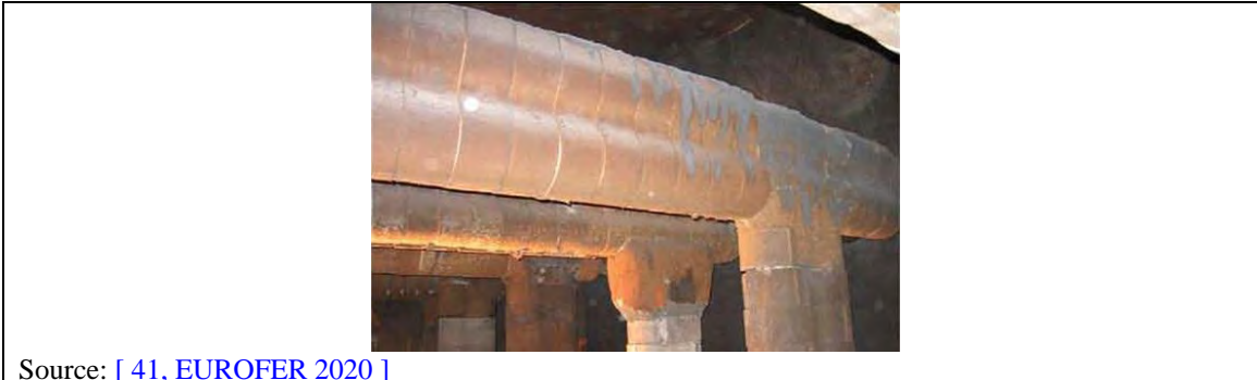
Figure 2.86: Double-pipes skid design for reheating furnaces
