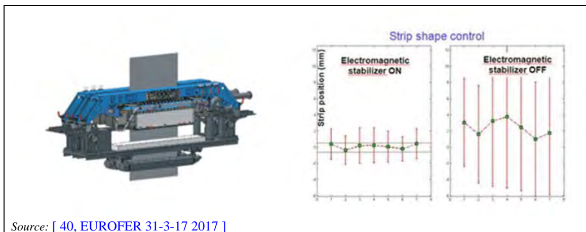
Figure 5.26: Schematic of an electromagnetic stabiliser
