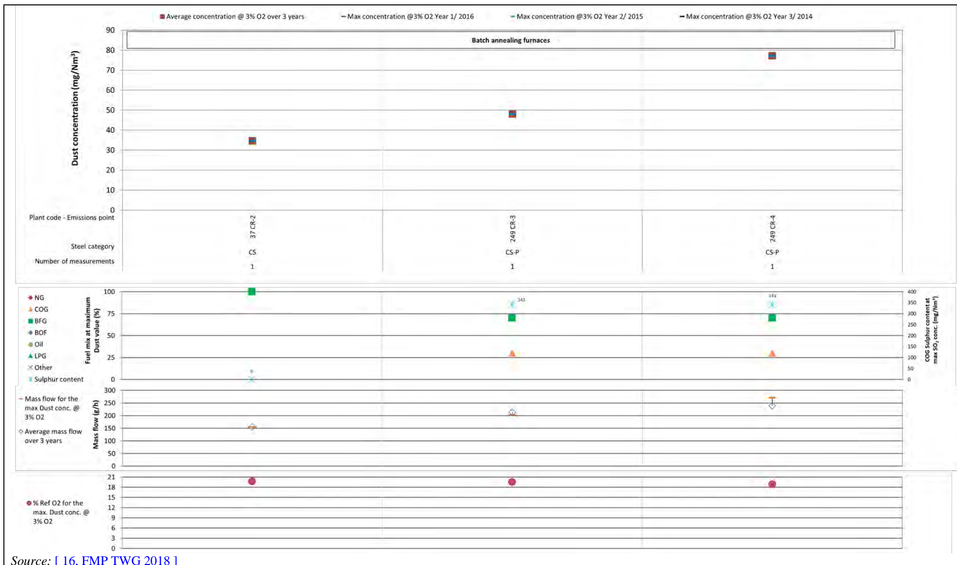
Figure 3.36: Dust emissions from feedstock heating (in mg/Nm 3 at 3 % oxygen) for fuels other than 100 % natural gas
