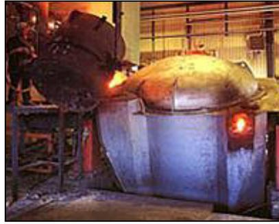
**Figure 2.16: Channel induction furnace**
