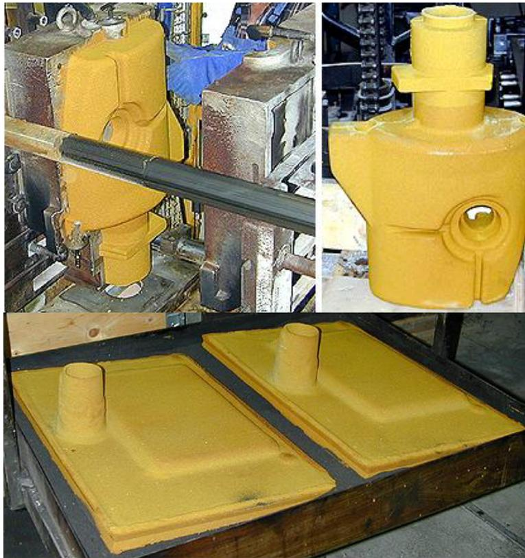
**Figure 2.33: Croning cores (top) and moulds (bottom)**
