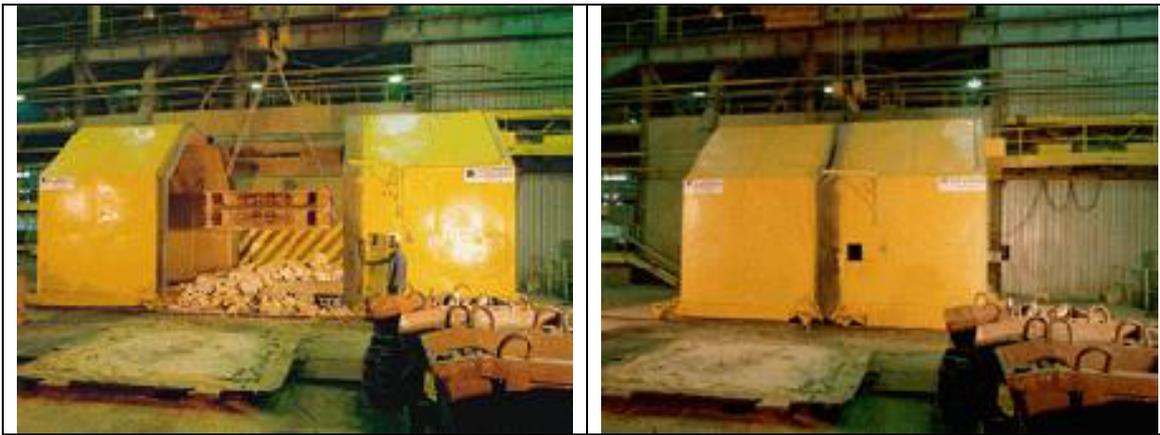
**Figure 4.17: Doghouse cover for a shake-out grate, for large-size batch castings**
