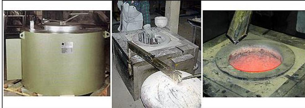
**Figure 2.20: Crucible furnaces**
