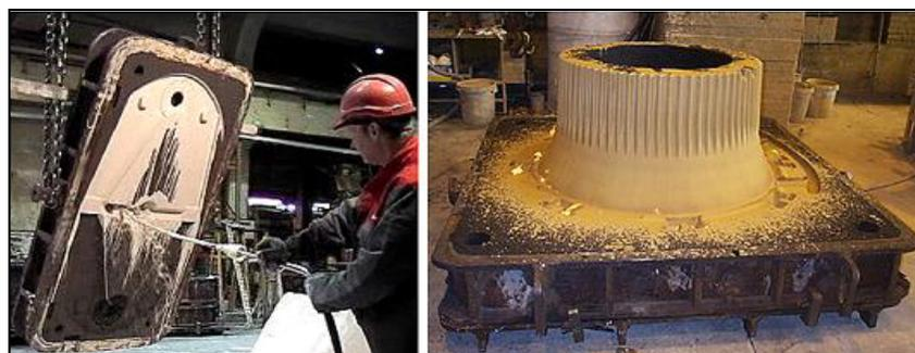
**Figure 2.34: Flow coating with alcohol-based coating, followed by firing or drying [237, HUT, 2003]**
