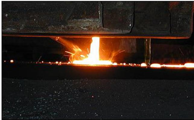
**Figure 2.24: Inoculation during pouring**
