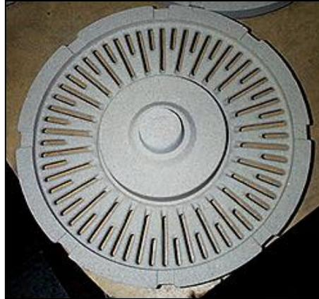
**Figure 2.32: Cold-box core**
