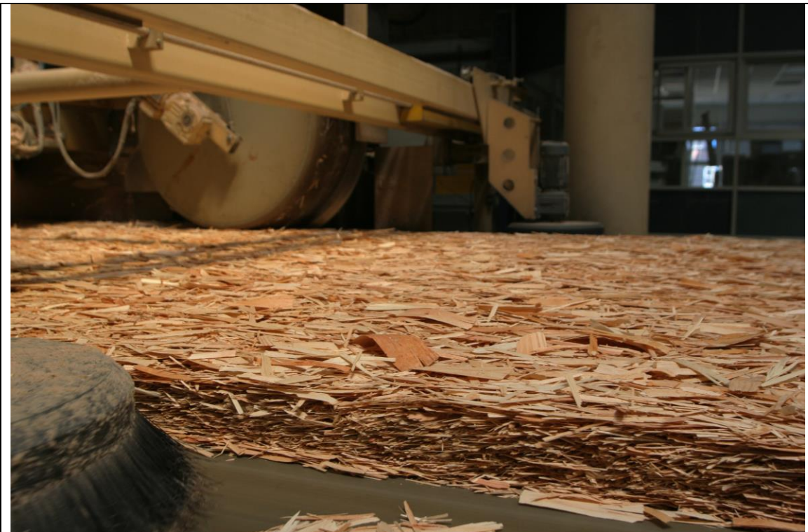
Figure 2.8: OSB mat after forming and trimming
