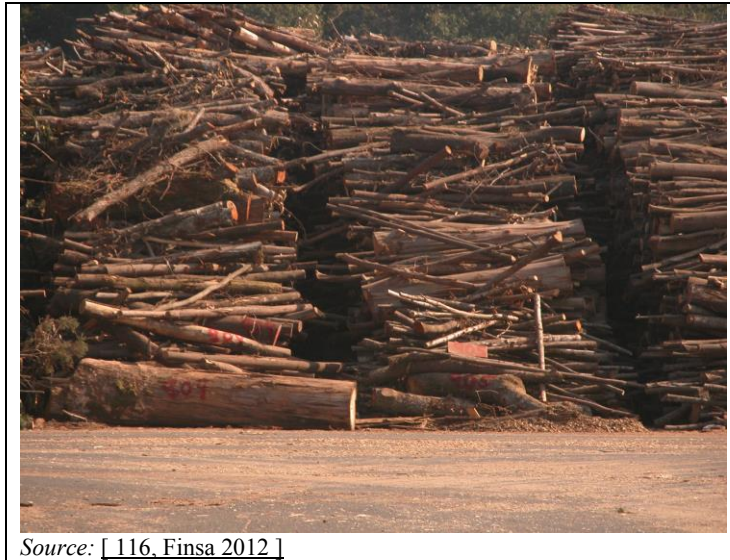
Figure 2.2: Storage of roundwood in a log yard
