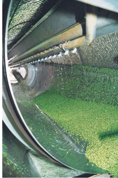
Figuur 18: Trommelwasser (website SALEENCO INDUSTRIES BVBA)
