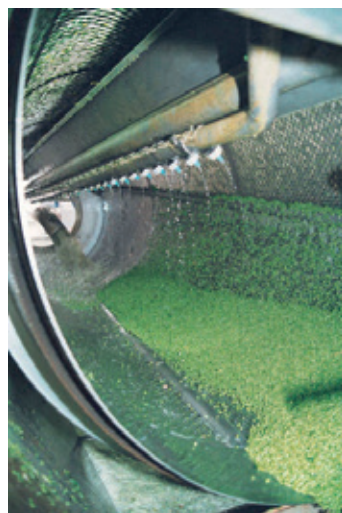
Figuur 18: Trommelwasser (website SALEENCO INDUSTRIES BVBA)
