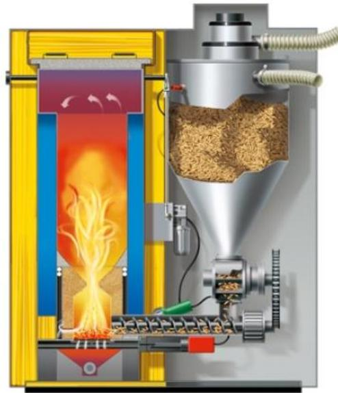
Figure 26: Pellet stove with automatic pellet feeding from an internal storage tank (Omniconfort, 2019)
