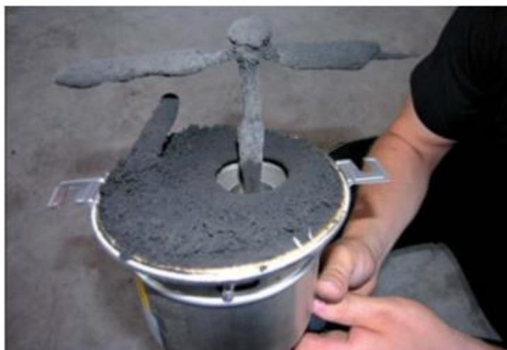
*Figure 34: Zumikon ESP electrode clamp, disassembled for cleaning after use (Hartmann, Turowski, & Kiener, 2010)*
