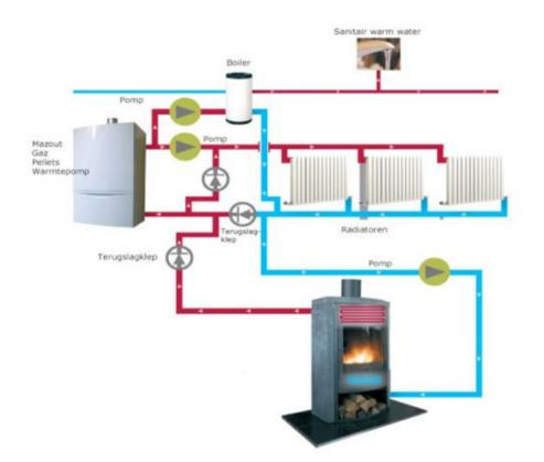
Figure 25: Example of connecting the hot flue gases to the central heating (return pipe in blue is optional) (DDG, 2019)
