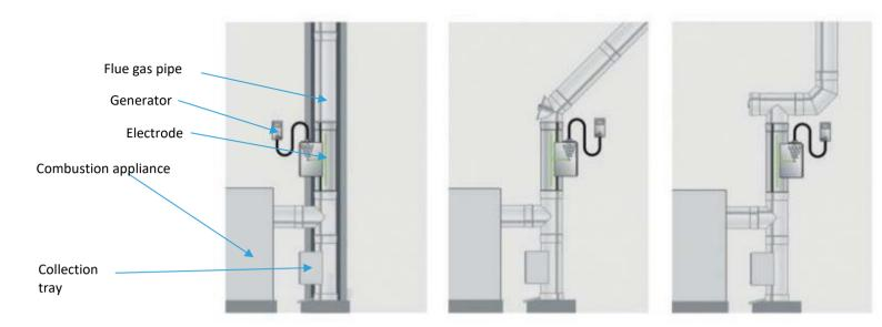
Figure 33: ESP fitted in the flue gas pipe (3 variants) (Supplier information electrofilter, 2019)
