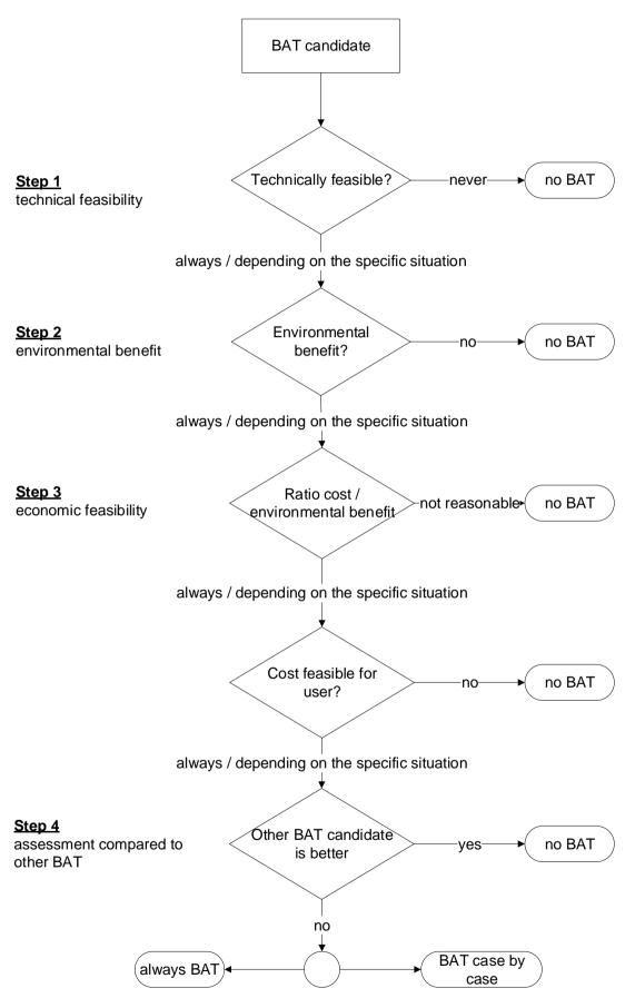
Figure 36: Selection of BAT based on scores for different criteria
