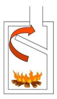
Figure 21: The flame baffle plate in the stove ensures that hot gases are not released directly up the flue gas pipe (Van Walsem Kachelspecialist, 2019)
