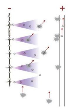
Figure 31: Operating principle of an ESP (Supplier information electrofilter, 2019)
