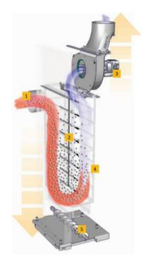
Figure 29: Operating principle of an integrated ESP in a pellet boiler (ETA Heiztechnik GmbH, 2019)
