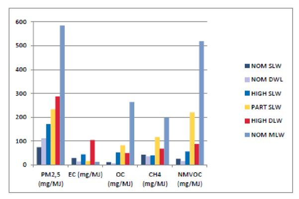
Figure 20: Average measured values when tested on 2 modern wood stoves (Kindbom, et al., 2017) (NOM = nominal load, HIGH = high load, PART = partial load, SLW = standard log wood, DLW = dry log wood, MLW = moist log wood)
