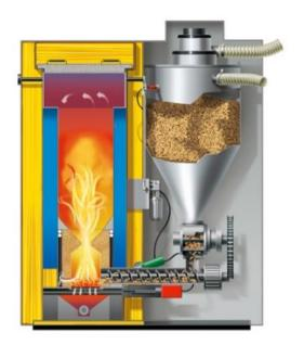
*Figure 26: Pellet stove with automatic pellet feeding from an internal storage tank* (Omniconfort, 2019)
