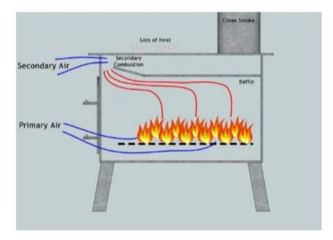
Figure 24: Schematic representation of a secondary combustion zone in a stove (Plomp, 2017)
