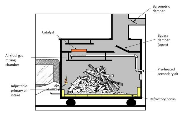
Figure 28: Ceramic catalytic wood combustion with bypass (Firecat, 2019)
