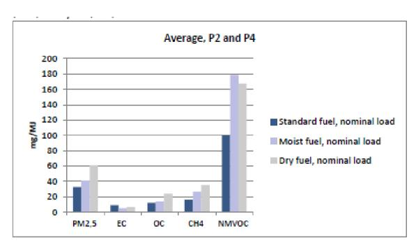
Figure 19: Average measured values when tested on 2 modern boilers fired with pieces of wood (Kindbom, et al., 2017)
