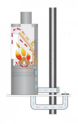
Figure 35: Illustration of an external air supply (blue arrows) for a wood stove (123-Kaminofen, 2019)
