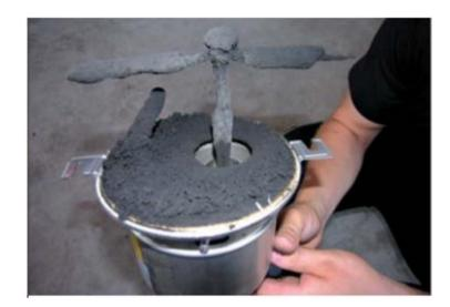
Figure 34: Zumikon ESP electrode clamp, disassembled for cleaning after use (Hartmann, Turowski, & Kiener, 2010)
