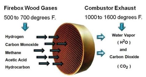
Figure 27: Operation of a catalyst and transformation of pollutants (Cork, 2013)
