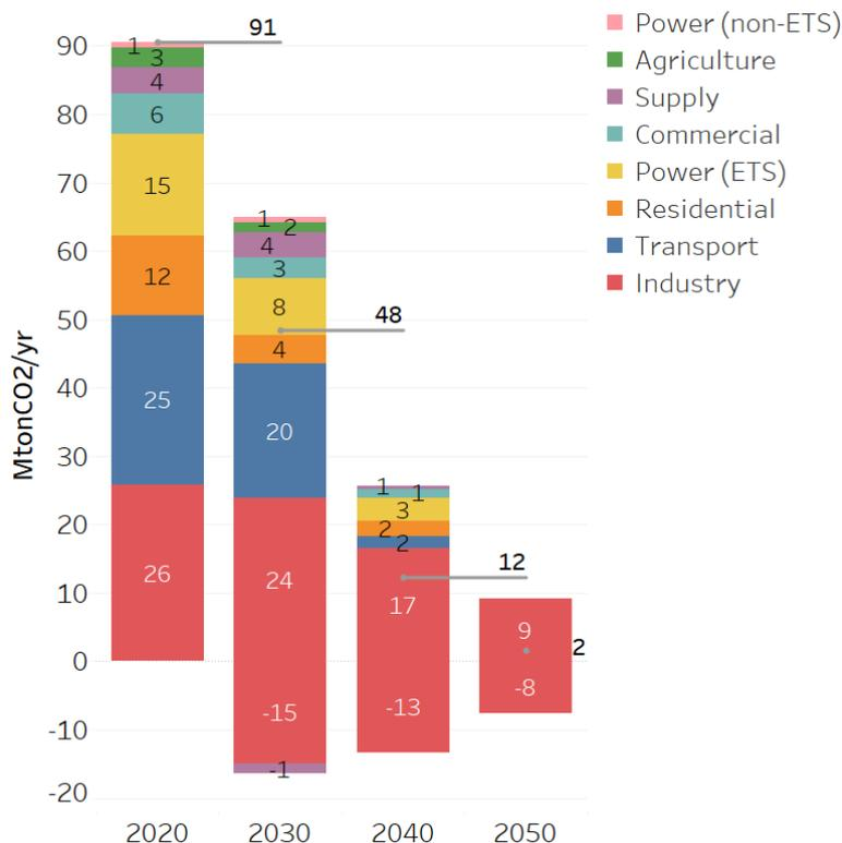
Figure 14: Annual CO<sub>2</sub> energy and process emissions in MtonCO<sub>2</sub> per year for SHIFT scenario. Net emissions indicated by lines. Note that the oil refineries are represented by the supply sector.
