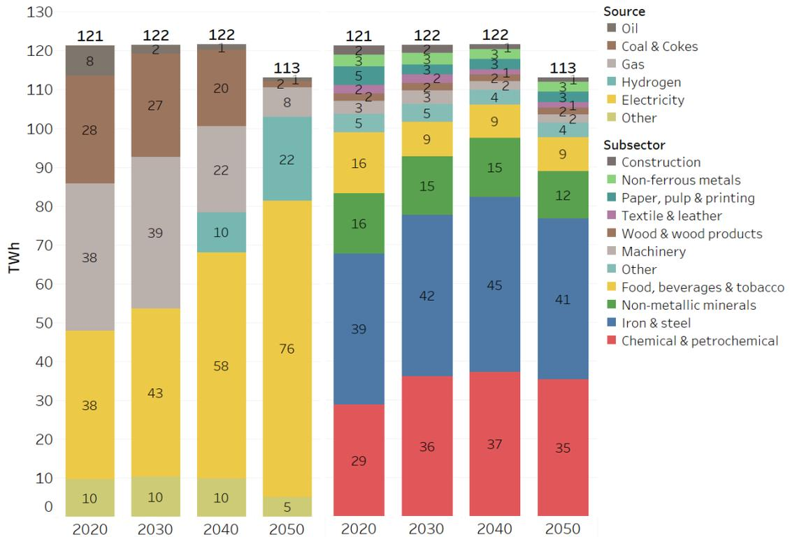
Figure 12: SHIFT scenario industry overview: final energy demand by source (left) and by subsector (right) in TWh. Note: Feedstock for industry is excluded in this graph.
