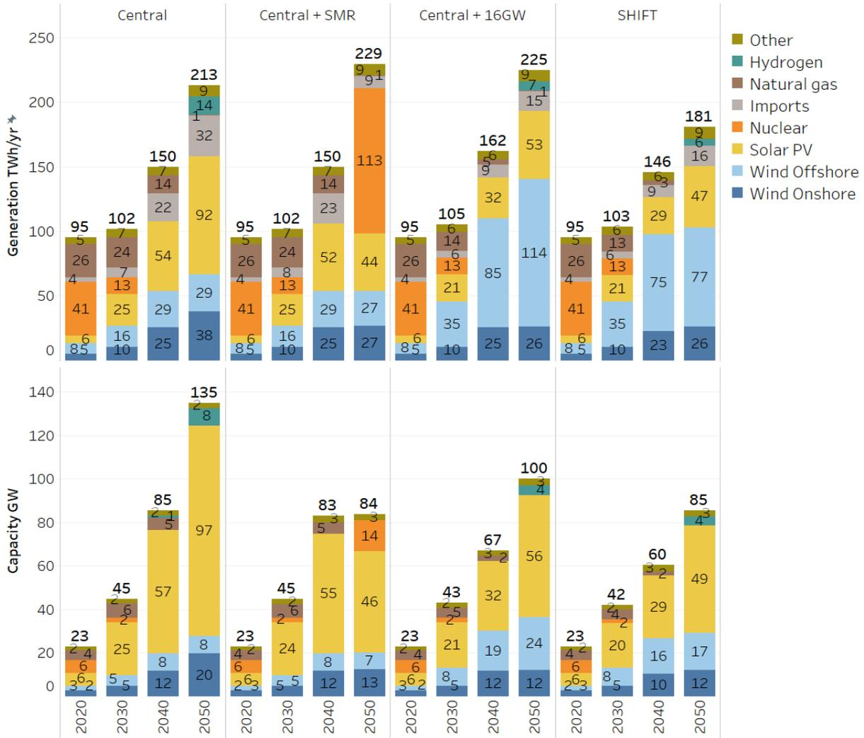
Figure 17: Power system comparison for capacity (bottom) and generation (top).
