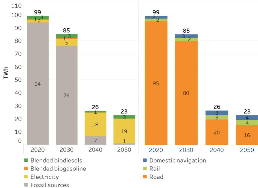
Figure 10: Transport sector SHIFT scenario: final energy consumption by energy source (left) and by modus (right).
