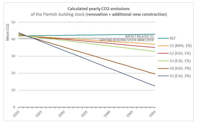
Figure 24. Calculated yearly CO2 emissions related to the Flemish building stock in case of different renovation scenarios, including additional new construction each year of 20.000 housing units.
