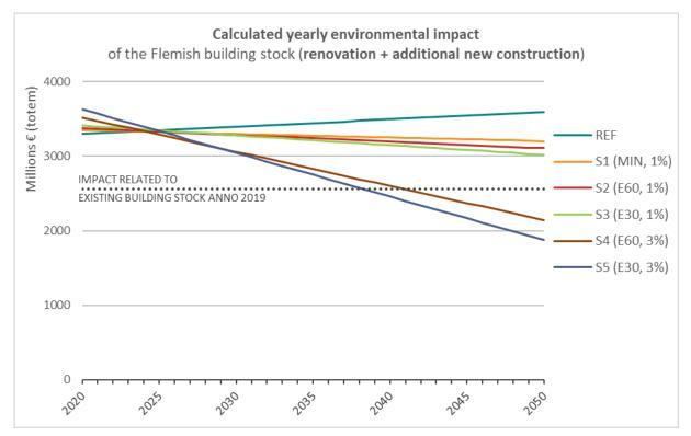
Figure 25. Calculated yearly monetised global environmental impact related to the Flemish building stock in case of different renovation scenarios, including additional new construction each year of 20.000 housing units.
