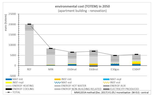
Considering the global environmental impact (Figure 10), the alternative with a heat pump has a higher impact because of the increased material related impact of technical installations (INST).
