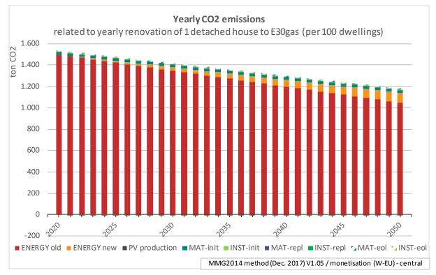
Figure 20. Yearly CO2 emissions related to a set of 100 detached buildings, considering the renovation of one house each year (1% renovation rate) according to the E30gas renovation scenario
