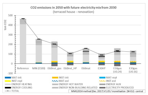
Figure 17. CO2 emissions generated by the terraced house over 30 years (from 2020 to 2050) for different renovation scenarios, with future electricity mix after 10 years
