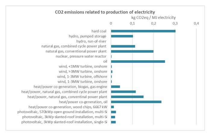
Figure 15. CO2 emissions related to the production of 1 MJ electricity produced by different power plants.
