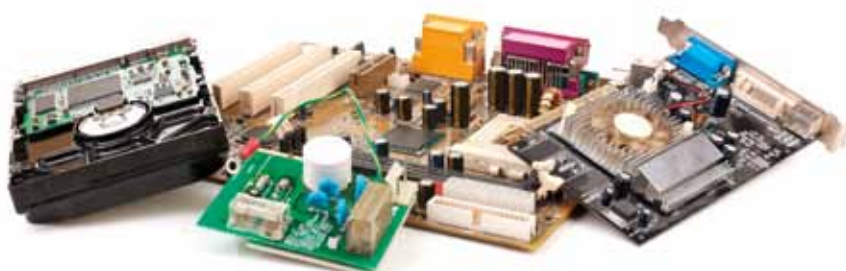
CRMRecovery is recovering of a range of critical raw materials from waste electrical and electronic equipment
