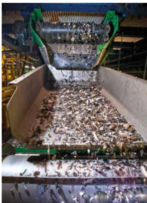
The shredded fraction represents around 20% of the weight of an ELV and contains valuable materials
