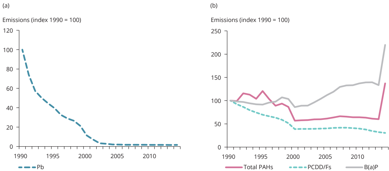
Figure 4.10 EU-28 emission trends in the sector group 'road transport' (a) for the priority HM Pb, and (b) for the POPs (PCDD/Fs, total PAHs and B(a)P between 1990 and 2014
