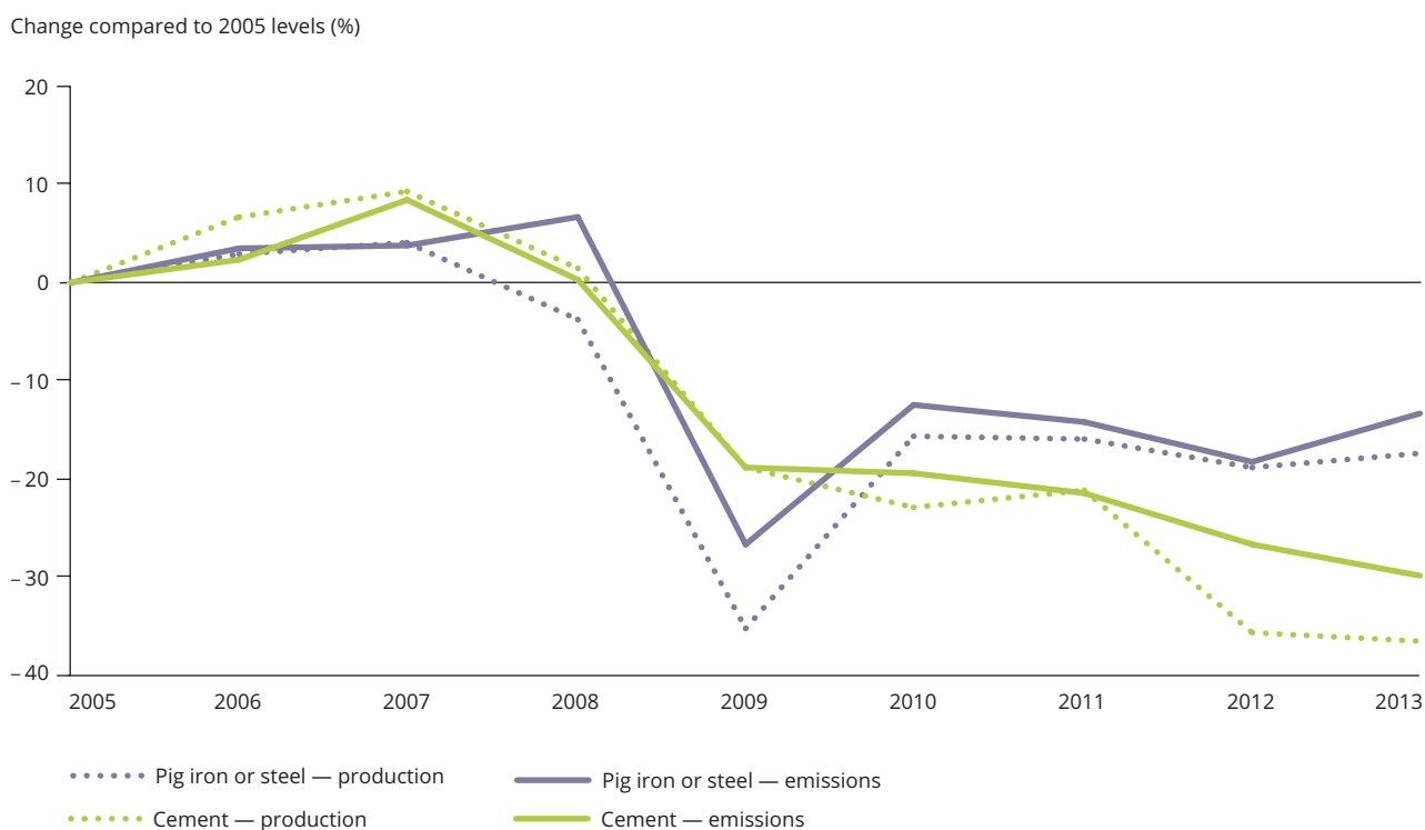
Figure 2.4 Comparison of production and emissions trends for pig iron or steel and cement, relative to 2005
