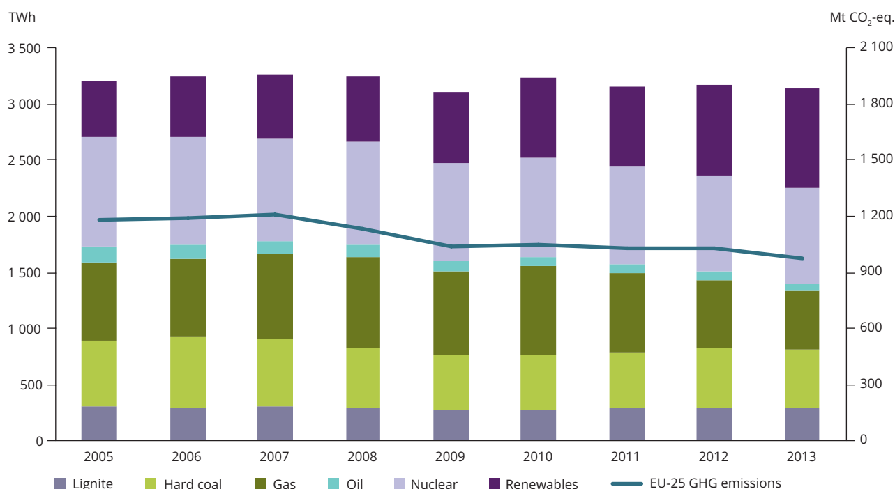
Figure 2.2 Gross electricity consumption by fuel in the EU-25, compared to ETS emissions from electricity generation
