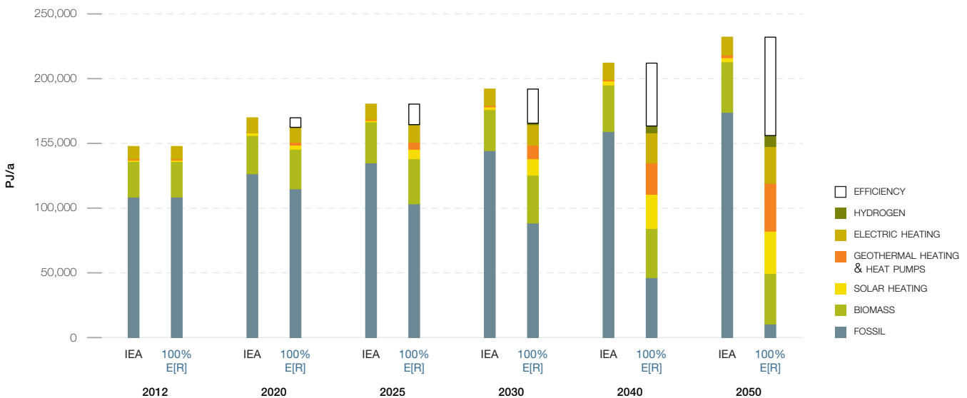
FIGURE 6 | PROJECTION OF HEAT SUPPLY BY SOURCE. IEA “CURRENT POLICIES” VERSUS 100% ENERGY [R]EVOLUTION
