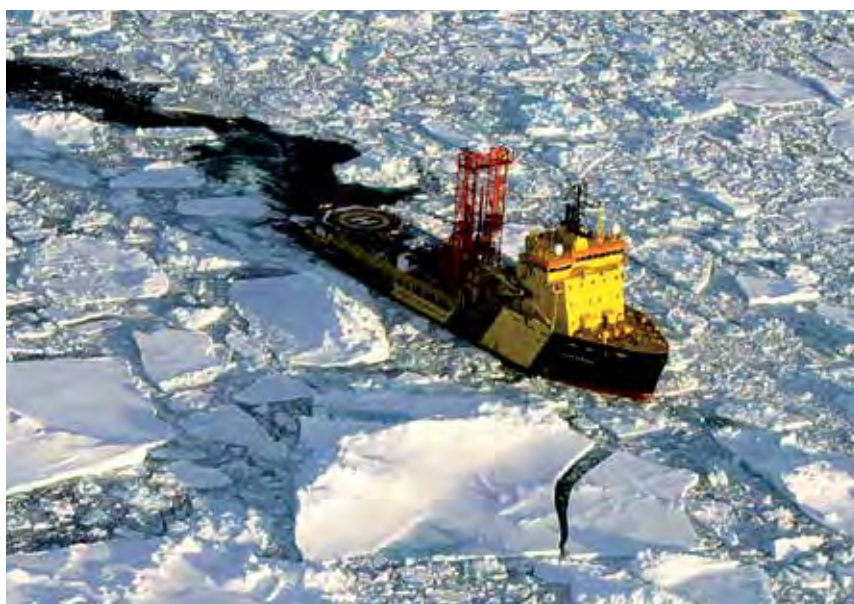
The drillship Vidar Viking in Arctic sea ice during an International Ocean Drilling Programme (IODP) Arctic coring expedition.
