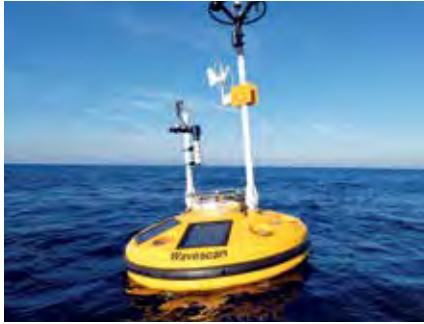
Ocean buoy and mooring for fixed-point measurements
