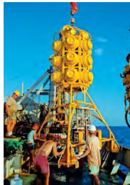
AlbeX Lander used for seafloor observation
