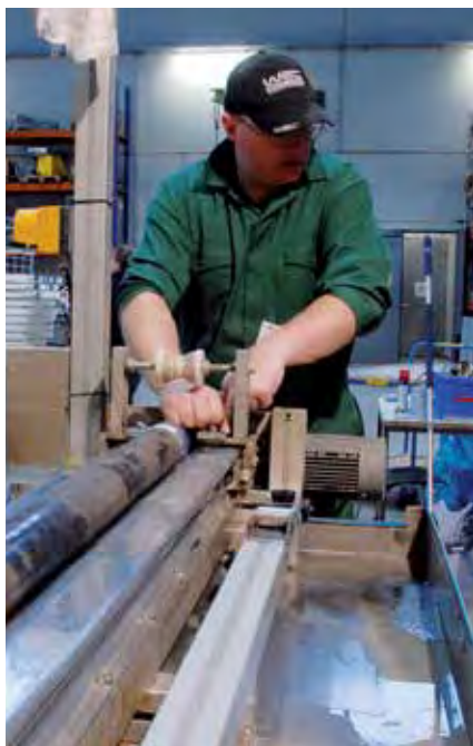
Core Splitting onboard an International Ocean Drilling Project research cruise.
