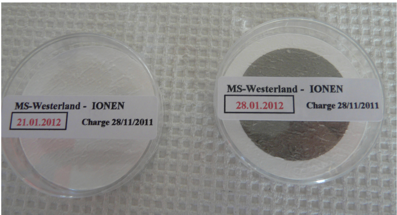
Figure 1.1 Carbonaceous compounds on a filter used to determine particulate matter mass concentrations with thermal-optical techniques
