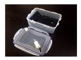
Berkeley Air PATS+ Zero Boxes are constructed by hand, on-site to fit the specific needs of PATS+ devices. Each box is air-tight and features a built-in HEPA filter to flush the box with clean, particle-free air, as well as a fitted one-way valve to prevent back-flow during the zeroing period. Zero boxes have been designed and lab tested with field conditions in mind, and are essential for zero calibration of particle-monitoring instruments in the field.
