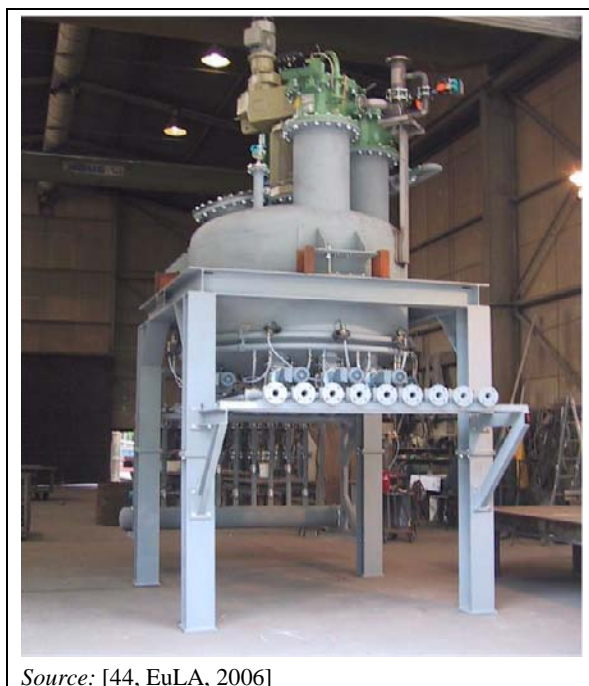
Figure 2.11: Example of a shaft kiln dosing system
