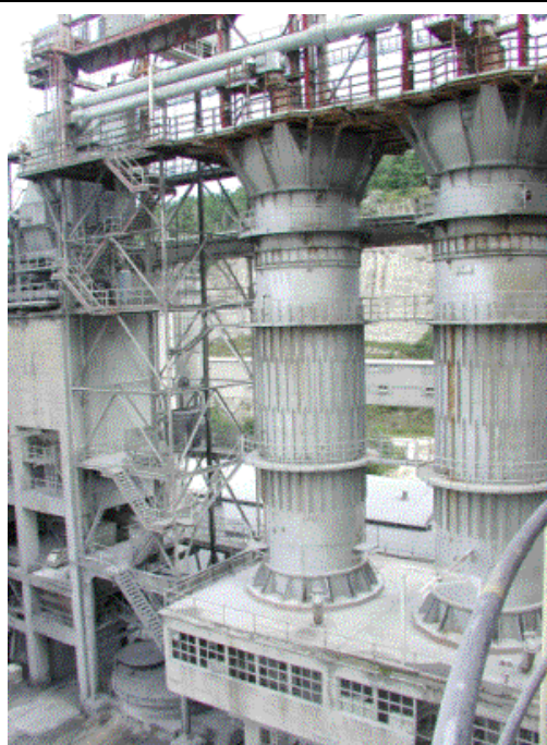
Figure 2.21: Mixed feed shaft kiln
