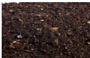
Figure 1.7: Hazardous waste – impregnated sawdust
