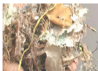
Figure 1.9: Specially prepared household waste used as fuel in cement kilns
