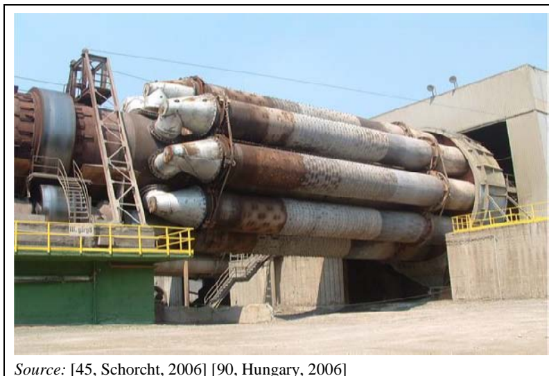
Figure 1.18: Example of a planetary cooler
