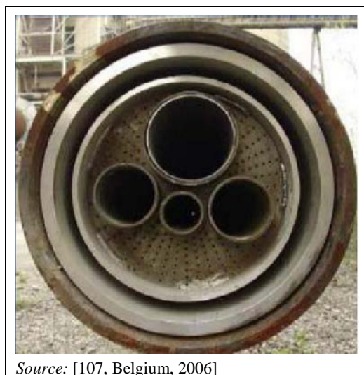
Figure 1.11: Example of a multi-channel burner
