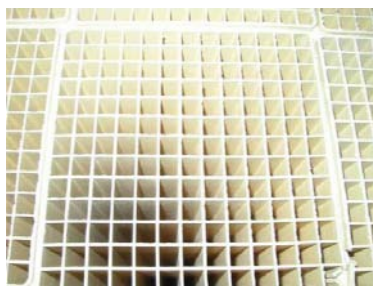
Figure 1.67: Example of an individual catalyst used for the SCR technique Source: [140, Italy, 2007]
