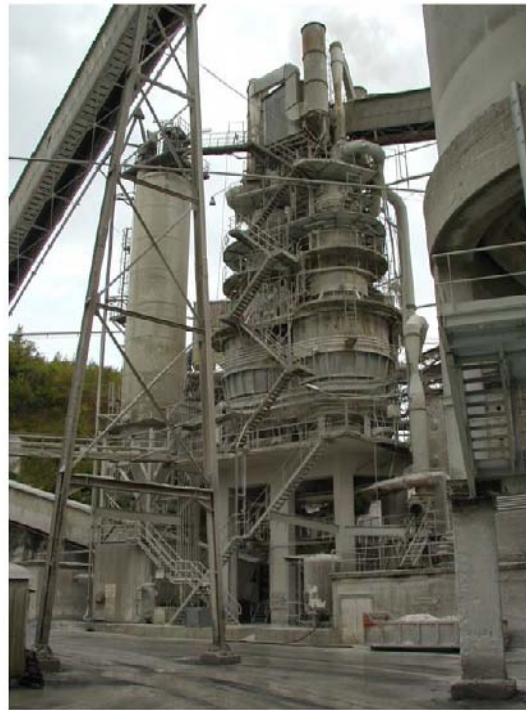
Figure 2.23: Example of a PFRK Source: [44, EuLA, 2006]
